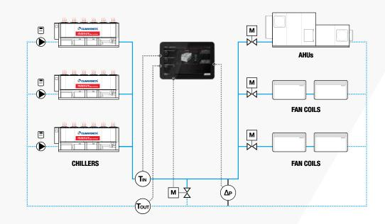
GROUP MANAGER C1 controls the primary chilled water and low temperature hot water pumps (CHW and LTHW) at variable flow, obtaining significant energy savings from the circulation of fluids.
